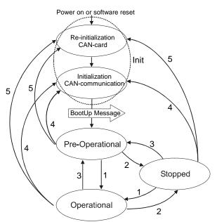
Fig. 1: CAN status diagram
